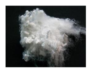
In particular the researchers found the way to treat cellulose (a material insoluble in usual solvents and inflammable) with nitric acid (nitrification), to dissolve the derivative with solutions of alcohol-ether, to prepare suitable extrusion devices (spinnerets) and finally to regenerate cellulose through saponification in alkaline baths (denitrification) in order to eliminate the danger inherent in the nitro compound (inflammable and explosive).
